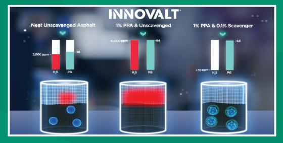
Asphalt binder modified with INNOVALT® Polyphosphoric Acid and Scavenger achieves the high temperature performance grade target while reducing hydrogen sulfide — **helping ensure a safe work environment**\*\*
