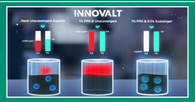
Asphalt binder modified with INNOVALT® Polyphosphoric Acid and Scavenger achieves the high temperature performance grade target while reducing hydrogen sulfide — **helping ensure a safe work environment**\*\*
