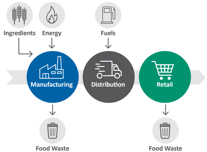
Figure 1. System Boundary Diagram for Downstream Gate-to-Grave LCA
